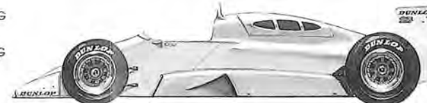
"DOME F-101" Manufactured in 1988; The first domestically manufactured full carbon composite body F3000 racing machine; It is the first stage of our F-1 racing program
